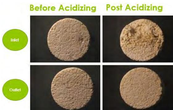
b. Face dissolution on Mount Gambier core sample at an acid concentration of 0.001 M HCl and injection rate of 3 cm<sup>3</sup>/min.
