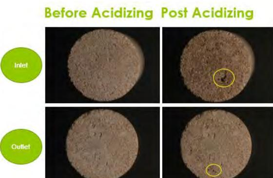
c. Single dominant wormhole on Indiana limestone core sample at an acid concentration of 0.1 M HCl and injection rate of 10 cm<sup>3</sup>/min.
