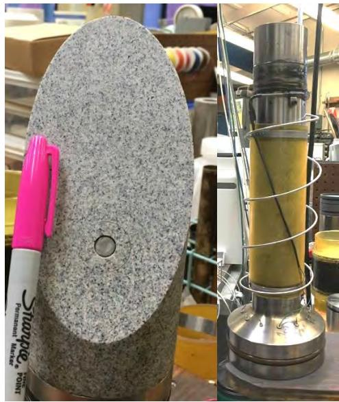
Figure 1. Left: Sawcut fault face with embedded pressure transducer. Right: Inverted sample assembly ready to place in pressure vessel. Coiled tubing provides pore pressure to end of granite sample (pore fluid must diffuse through granite to reach fault). Pressure transducer is embedded in lower sample half.
